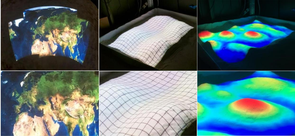
Figure 1 Left: Result of our system using 3 projectors and 3 cameras on a hemisphere. Middle: Showing our result projecting on a sand pit with 4 projectors and 4 cameras. The projected grid shows the accuracy of registration in the overlap area of the projectors. Right: A seamless elevation map projected on an arbitrary shape of sand pit. Note that warmer colors light higher regions and cooler colors for lower parts demonstrating the accuracy of surface geometry reconstruction.
